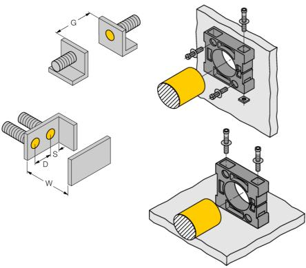
The given minimum distances have been checked in compliance with the standard switching distance. Should the sensitivity of the sensors be changed via potentiometer, the data sheet specifications no longer apply.
