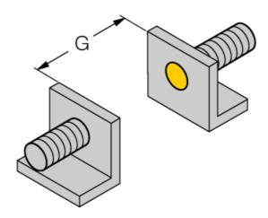
The given minimum distances have been checked in compliance with the standard switching distance. Should the sensitivity of the sensors be changed via potentiometer, the data sheet specifications no longer apply.
