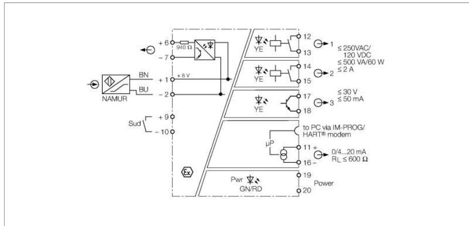
The rotation speed monitor IM21-14EX-CDTRI monitors frequencies, rotation speeds and pulse trains of rotating motor, gear or turbine parts according to over or undershoot of adjusted limit values. A display at the front indicates the current value.
