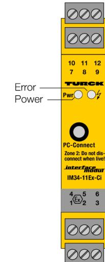
The 1-channel Ex-temperature measuring amplifier IM34-11EX-CI is designed to evaluate the temperature-dependent variations of resistance thermo detectors (RTD) Ni100/Pt100, thermoelement types B, E, J, K, L, N, R, S and T or low voltages in a range of -160...+160 mV and to output them as linear temperature current signals 0/4...20 mA.
