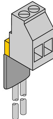
The resistor module meets the requirements for line monitoring between a mechanical contact and a signal processor. The input circuit is designed for sensors according to EN60947-5-6 (NAMUR) and is equipped with a wire-break and short-circuit monitoring function.
