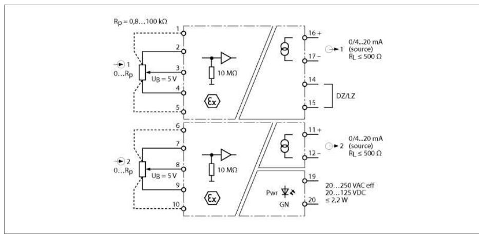
The 2-channel potentiometer amplifier IM36-22EX-I separates signals from 3-wire or 5-wire potentiometers and transfers these as standard 0/4...20 mA analog signals from the Ex area to the non-Ex area. Live-zero operation is activated for both channels through bridging terminals 14 and 15. The resistance value of the wiper contact is collected and processed linearly in a range between 0  $\Omega$  and the potentiometer's end value (see fig.).
