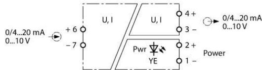
Standard, active voltage or current signals are galvanically isolated, transmitted and converted to other signal types via the 1-channel universal analog data transmitter IMS-AI-UNI/24VDC.
