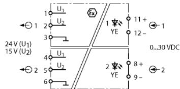
The solenoid drivers of series IM72-22EX/L feature an intrinsically safe output with limited current and voltage. Thus making direct connection to loads in the Ex-area possible.
