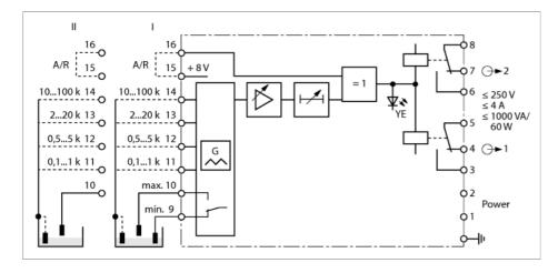
The 1-channel level control MS91-12-R monitors and regulates conductive liquid levels (II). As a dual level regulator, it can be used to control pumps and solenoid valves (I). As monitoring device it is designed for run-dry or over flow protection.
