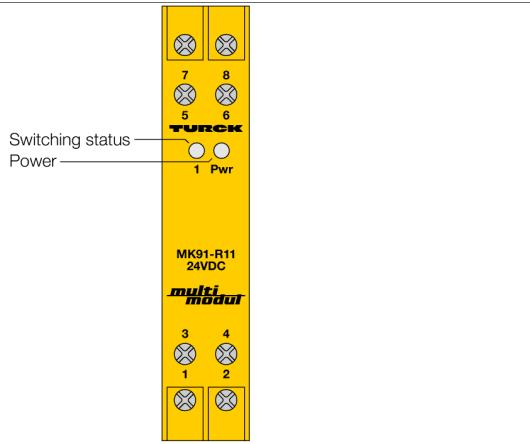
The 1-channel level control MK91-R11/24VDC regulates conductive liquid levels. Electrodes connected to the device analyse the resistance of the liquid against the body of the container.
