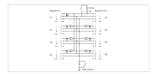
The 6-channel Ex junction box JBBS-49SC-E613/3G is designed for FOUNDATION™ fieldbus systems.
