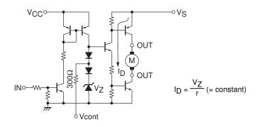
As shown in the above diagram, the V cont pin outputs the voltage of the band gap Zener V<sub>Z</sub> + V<sub>F</sub> (=1.93V). In normal use, this pin is left open.
