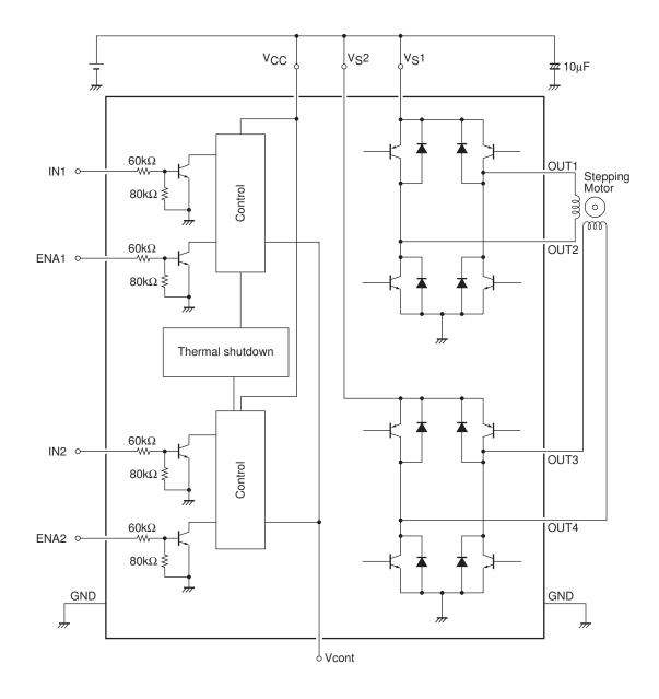
\* : As long as the voltages applied to V<sub>CC</sub>, V<sub>S</sub>1, V<sub>S</sub>2, ENA1, ENA2, IN1 and IN2 are within the limits set by the absolute maximum ratings, there are no restrictions on the relationship of each voltage level in comparison with the others (regarding which is higher or lower). (ex. V<sub>CC</sub> = 3V, V<sub>S</sub>1, 2 = 2V, ENA = IN = 5V)
