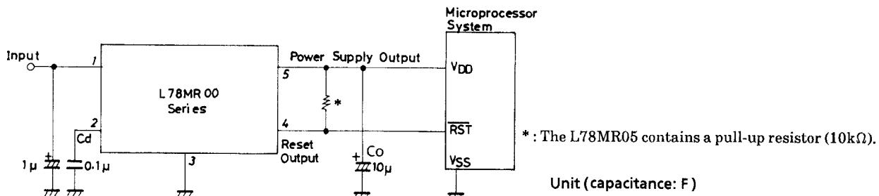
Note on use) If a load current (in particular, pulse-like load current) that is greater than a rated value is used, a reset signal may be generated due to the overload. Please keep it in mind.
