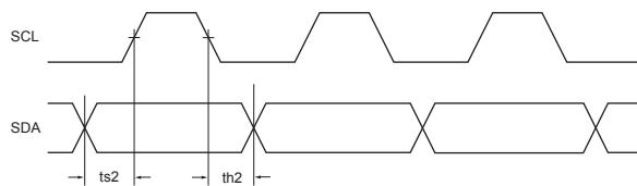
When data is not being transferred, both SCL and SDA are set in the "H" state.
