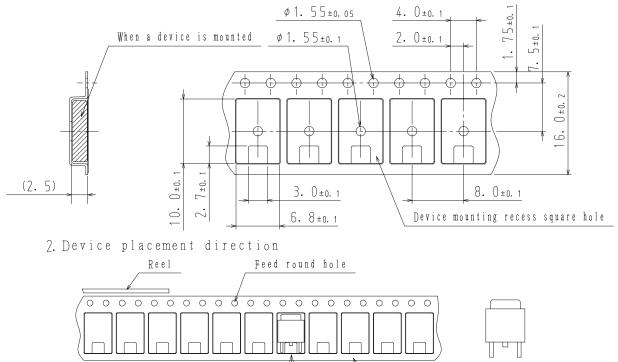
T Those with one electrode terminal on the feed hole side ..... TL
