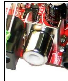
The + signal is lead to the middle of the connector. The outside part is the GND.
