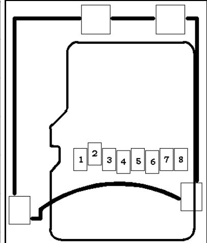
Notice that the pad numeration is written at the bottom of OLinuXino-MINI under the microSD
