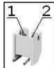
The pins are also written on the top of the board in the base of the connector.
