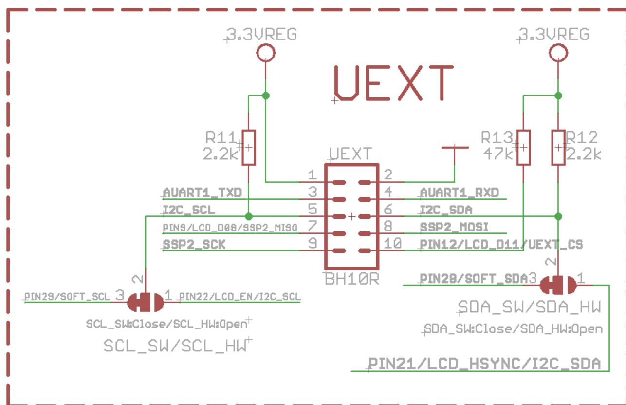
\*Note the two jumpers PIN29/SOFT\_CL – PIN22/LCD\_EN/I2C\_SCL, and PIN28/SOFT\_SDA3 – PIN21/LCD\_HSYNC/I2C\_SDA which by default are set to a software SPI. They can be used to set the whole UEXT to a hardware SPI.
