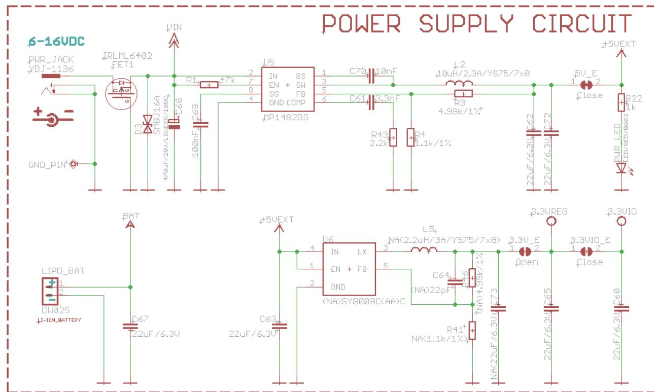
Note that the whole 3.3V part is not mounted (elements marked as NA) by default because we use the internal 3.3V DC-DC convertor in the iMX233. However, the internal DC-DC in the processor is not very reliable when a lot of current is required. It is better to mount the elements of the 3.3V part circuit if you wish to use 3.3V at heavier loads.
