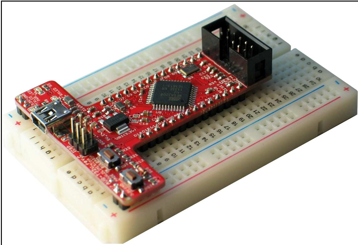
If you want to upgrade the bootloader, or program the board without the ARDUINO-IDE there are pinouts for ICSP programmer (note that there IS a 6-pin connector mounted). You can use our AVR-ISP-ISO, or AVR-ISP-TINY programmer for custom programming without ARDUINO IDE.
