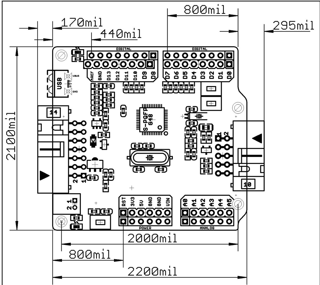
The three highest elements on the board with same height are: JTAG/SBW connector – 340mil; UEXT connector – 340mil; Arduino shield connectors – 340mil.
