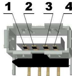
**USBM0** and **USBP0** form the differential input/output of the USB host 0.
