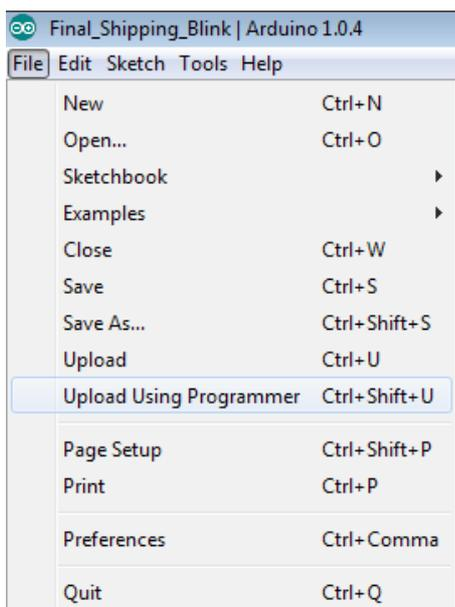
Special mention for Olimex boards – sometimes the board refuses to reset before programming when using Arduino. Try holding the reset button and release it simultaneously while clicking “Upload Using Programmer”.
