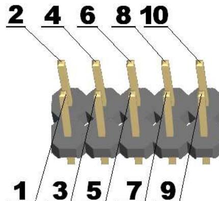
The **JTAG** connector is 2x5 pin with 0,1" step and Atmel's compatible layout. The PIN.1 is marked with square pad on bottom and arrow on top.
