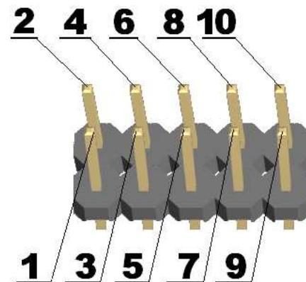
The **ICSP** connector is 2x5 pin with 0,1" step and Atmel STKxxx compatible layout. The PIN.1 is marked with square pad on bottom and arrow on top.
