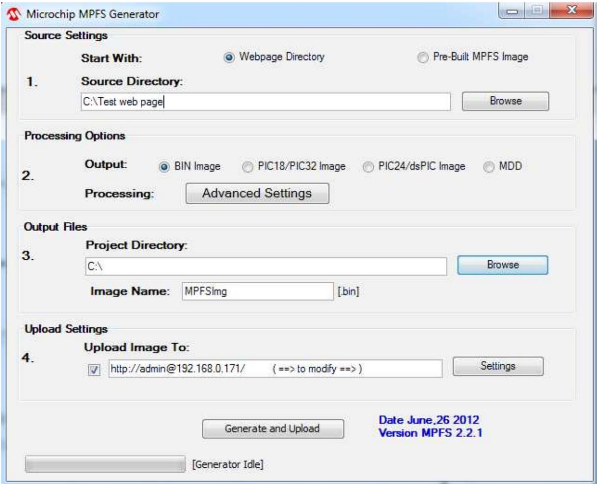
A very handy feature of the utility is point 4, which may be used to automatically upload the image to the board after a successful conversion. Enter the IP of your board and leave the other fields at defaults. Press the
