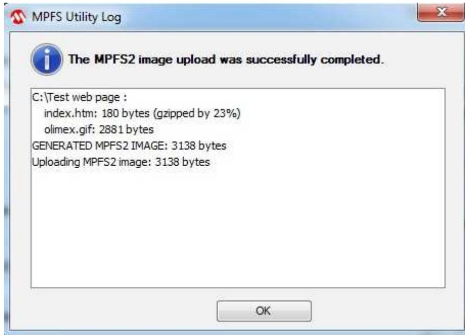
Please note that an image file (in this case MPFSImg.bin) is generated and may be used later if you select the 'Pre-built MPFS image' radio button at the top of the utility program window.
