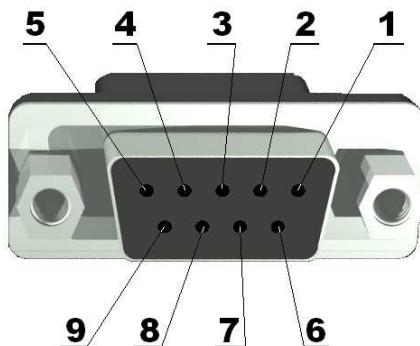
**TXD** **Output Transmit Data.** This is the asynchronous serial data output (RS232) for the shift register on the UART controller.
