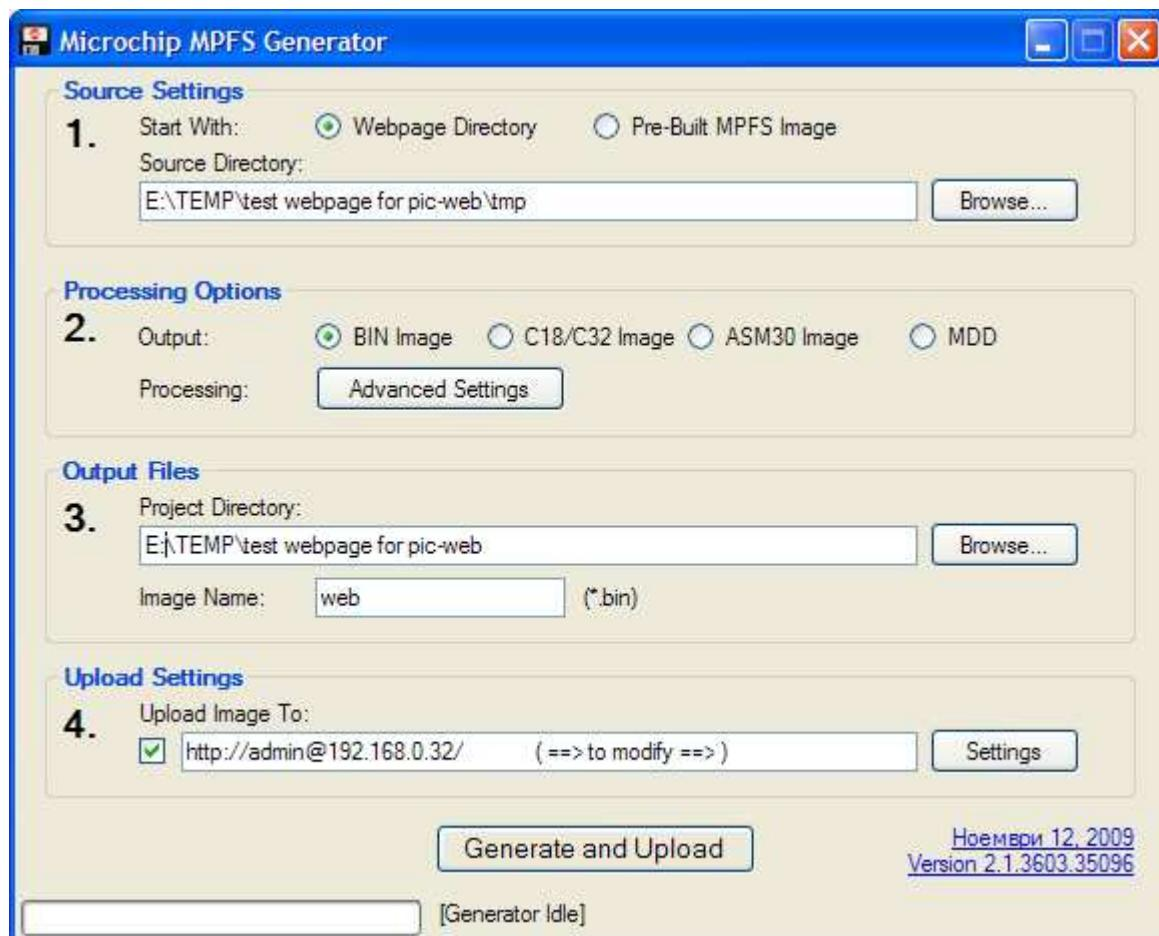
A very handy feature of the utility is point 4, which may be used to automatically upload the image to the board after a successful conversion. Enter the IP of your board and leave the other fields
