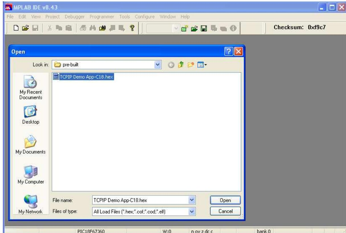
For programming the PIC just push the program button on the tools or selecting the menu Programmer -> Program.
