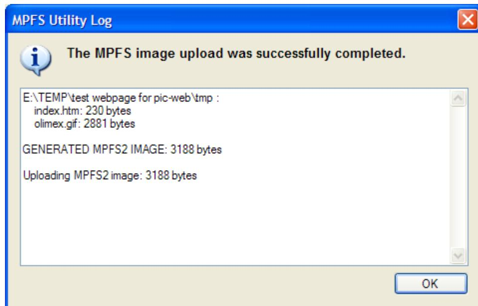
Please note that an image file (in this case web.bin) is generated and may be used later if you select the 'Pre-built MPFS image' radio button at the top of the utility program window.
