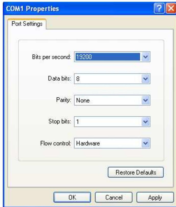
These are the basic steps to configure the connection. If you want to see what you are typing you should set the checkbox “Echo typed characters locally” in File->Properties->Settings->ASCII Setup. Then save the connection for later use.
