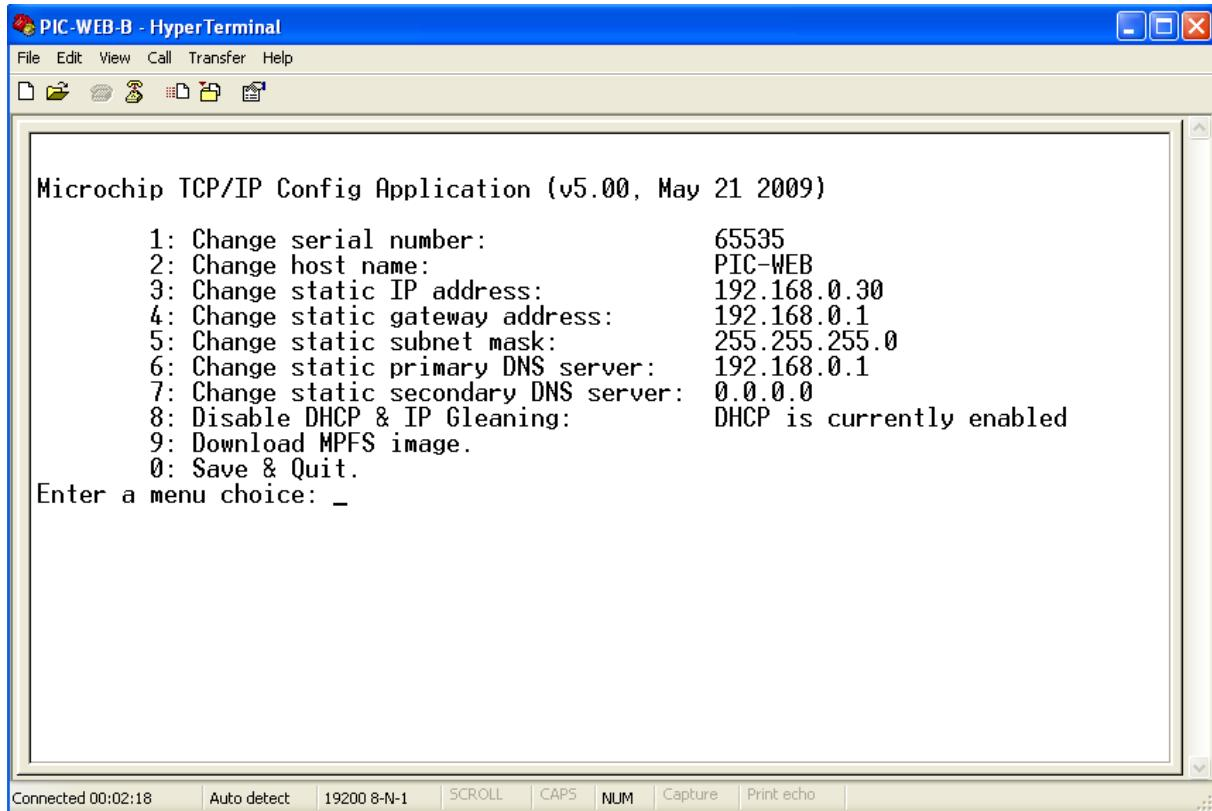
The third option allow you to change the board IP number. Just type 3, then enter the new IP compatible with your local network configuration. After that push ENTER and return to the main menu again.
