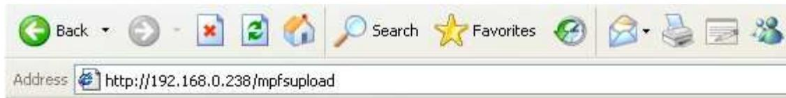
Click on the button “Choose File” to select the “\*.bin” file you are about to upload. Select the image file in directory .\PIC\_WEB\_RevB\_Patch\pre-built\MPFSImg2.bin and press ‘Upload’. Sit back and relax while the upload takes place and then navigate to the home page to behold the page just uploaded.
