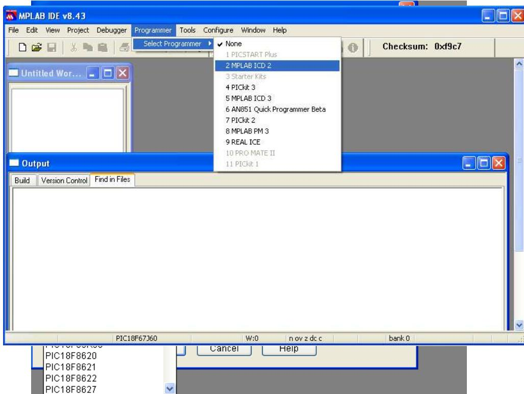
Wait while MPLAB is downloading operation system, and after ICD2 is connected – check in menu Programmer – Settings – Power – there is option – Power target circuit from MPLAB ICD 2 –
