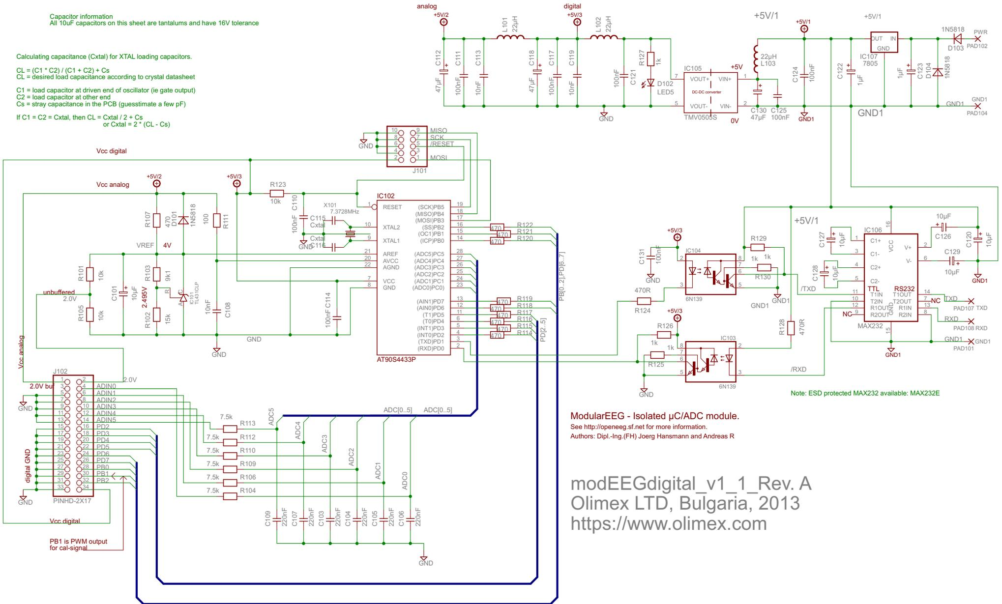
ModularEEG - Isolated  $\mu$ C/ADC module.
