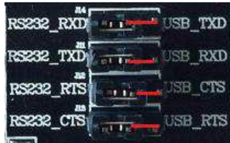
Figure 5: USB to serial jumper connect
