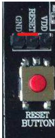
Figure 9: Jumper setting for low effective RESET
