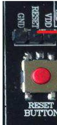
Figure 8: Jumper setting for high effective RESET
