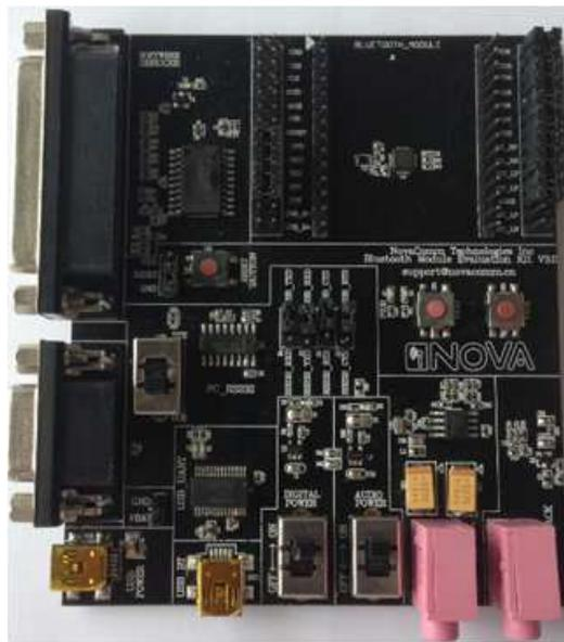
Figure 1: Evaluation Kit Main Board: ABBTM-NVC-MB-EVK
