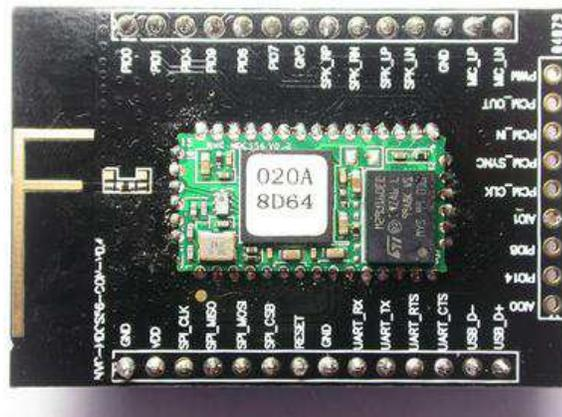
Figure 17: ABBTM-NVC-MDCS56-CON (49 x 33.5mm)
