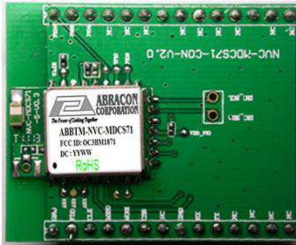
Figure 16: ABBTM-NVC-MDCS71-CON (41 x 33mm)
