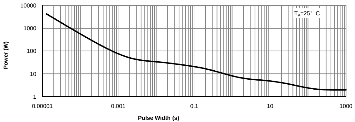
Figure 14: Single Pulse Power Rating Junction-to-Ambient (Note H)
