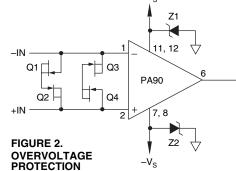
reversals to ground. Whether the zeners are used or not, the system power supply should be evaluated for transient performance including power-on overshoot and power-off polarity reversals as well as line regulation.
