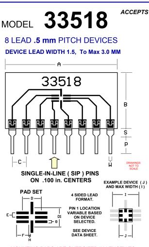
MOUNTING PADS ARE OVERSIZED IN LENGTH TO ACCEPT A WIDER RANGE OF DEVICE WIDTHS AND TOLERANCES AND TO PERMIT HAND SOLDERING. SEE WEBSITE FOR SOLDERING SUGGESTIONS
