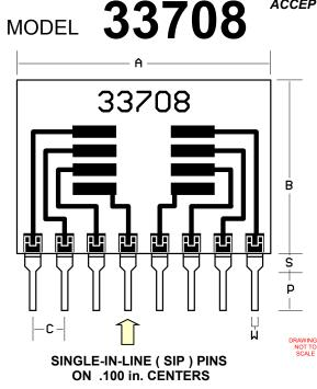
FXAMPLE DEVICE (J) PAD SET AND MAX WIDTH (1)
