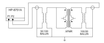
4. Crosstalk Attenuation — In the dual packages, which contain transmit and receive transformers side by side, sufficient crosstalk attenuation is achieved by the inherent characteristics of the toroid cores as well as by their proper positioning. The crosstalk attenuation is typically 50 dB or better from 100 kHz to 10 MHz. This result was established with the test circuit shown below.
