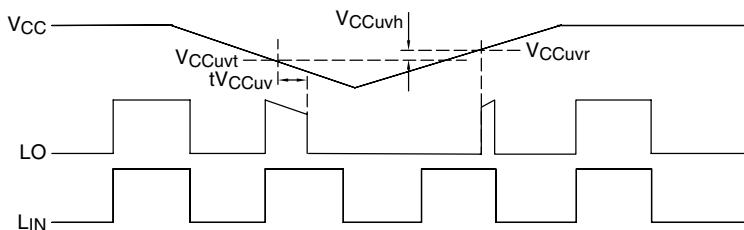
When  $V_{CC}$  supply voltage keeps lower UV trip voltage ( $V_{CCuvt} = V_{CCuvr} - V_{CCuvh}$ ) for  $V_{CC}$  supply UV filter time, output signal becomes “L”. And then, when  $V_{CC}$  supply voltage is higher than UV reset voltage, input signal ( $L_{IN}$ ) is “L”; output signal  $HO$  becomes “H”.
