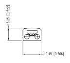
\*UNLESS OTHERWISE SPECIFIED TOLERANCES PER DECIMAL PRECISION ARE: X=±1 (±0.039), X.X=±0.5 (±0.020), X.XX=±0.25 (±0.010), X.XXX=±0.127 (±0.005). LEAD SIZE=±0.05 (±0.002), LEAD LENGTH=±0.75 (±0.030). MIN=  $^{+DECIMAL}_{-0.00}$  PRECISION MAX.=  $^{+0.00}_{-DECIMAL}$  PRECISION
