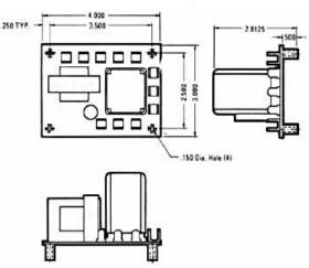
Control Relay: Plug-in Type with Dust-Tight Cover
