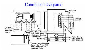
Model LCT is a forward mode control. The control relay is energized when liquid rises to contact the "H" probe. The time delay on operate is 3 seconds nominal and 0.5 seconds on release. Other values between 0.5 and 10 seconds are available on request. The control relay is pulled in and remains energized until liquid drops below the "L" probe. Sensitivity is adjustable.
