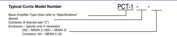
The composite number above reads as a "PCT amplifier for 120VAC supply without contactor and less enclosure." Contact factory for additional information.
