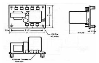
This is a fixed-sensitivity, forward mode control. The control relay is energized when liquid rises to contact the "H" probe. The control relay is pulled in and remains energized until liquid drops below the "L" probe.
