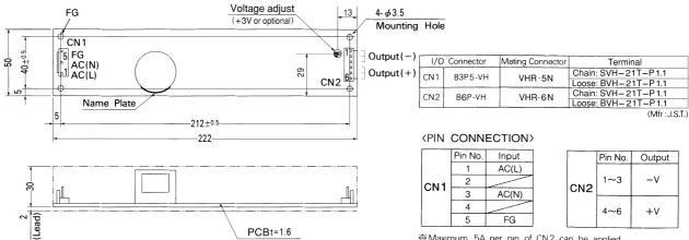
⅔Maximum 5A per pin of CN2 can be applied
