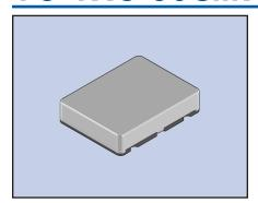
The VC-TXO-39SMX is a VC (Voltage Controlled) **FEATURES** TCXO (Temperature Compensated Crystal Oscillator) featuring very tight stability over a wide temperature range. The small SMD ceramic package measures 11.4 x 9.6 x 2.3 mm. The voltage control has a tuning range of  $\pm$  12 ppm typical. The low profile package is ideal for wireless communications applications.
