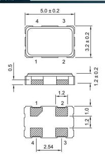
PAD FUNCTION: 1:ENABLE CONTROL 2:GND 3:OUT 4:VDD
