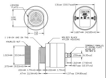
NOTE A: TERMINALS-032 BRASS TIN PLATED, TAPPED FOR #6-32 SCREW. TWO #6-32 NICKEL PLATED BRASS SCREWS INCLUBED. WILL ACCEPT 1/4' QUICK CONNECT. NOTE B: MDUNTING- REMOVE BLACK PLASTIC NUT AND INSERT THREADED FRONT THROUGH 1.25' HOLE PUNCHED IN PANEL, IF DRIENTATION IS NEEDED, NOTE LOCKING FLATS ON DRAVING, SCREW NUT BACK ON. DO NOT OVERTIGHTEN.
