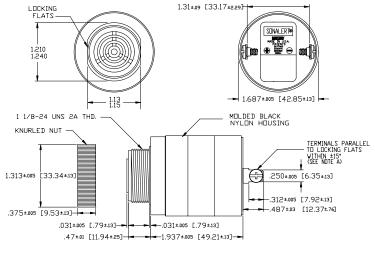
NOTE A: TERMINALS-032 BRASS TIN PLATED, TAPPED FOR #6-32 SCREW. TWO #6-32 NICKEL PLATED BRASS SCREWS INCLUBED. WILL ACCEPT 1/4' QUICK CONNECT. NOTE B: MOUNTING- REMOVE BLACK PLASTIC NUT
