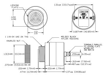
NOTE A: TERMINALS-.032 BRASS TIN PLATED, TAPPED FOR #6-32 SCREW. TWO #6-32 NICEL PLATED BRASS SCREWS INCLUDED, WILL ACCEPT 1/4\* QUICK CONNECT. NOTE B: MOUNTING- REMOVE BLACK PLASTIC NUT AND INSERT THREADED FRONT THROUGH 125' HOLE PUNCHED IN PANEL, IF DRIENTATION IS NEEDED, NOTE LOCKING FLATS ON DRAWING. SCREW NUT BACK ON. DO NOT OVERTIGHTEN.
