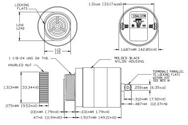
NOTE A: TERMINALS-.032 BRASS TIN PLATED, TAPPED FOR #6-32 SCREW. TWO #6-32 NICKEL PLATED BRASS SCREWS INCLUBED. WILA ACCEPT 1/4' QUICK CONNECT. NOTE B: MOUNTING- REMOVE BLACK PLASTIC NUT AND INSERT THREADED FRONT THROUGH 125' HOLE PUNCHED IN PANEL, IF DERENTATION IS NEEDED, NOTE LOCKING FLATS ON DRAVING. SCREW NUT BACK ON. DO NOT OVERTIGHTEN.
