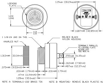
NOTE A: TERMINALS-032 BRASS TIN PLATED, TAPPED FOR #6-32 SCREW. TWO #6-32 NICKEL PLATED BRASS SCREWS INCLUDED. WILL ACCEPT 1/4' GUICK CONNECT.
