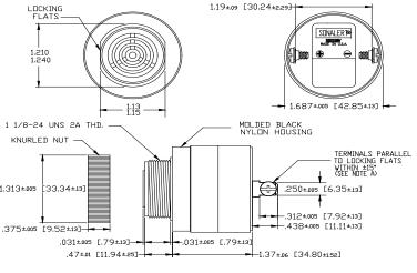
NOTE A TERMINALS-.032 BRASS TIN PLATED, TAPPED FOR #6-32 SCREW. TWU #6-32 NICKEL PLATED BRASS SCREWS INCLUDED. WILL ACCEPT 1/4" QUICK CONNECT. NOTE B: MOUNTING- REMOVE BLACK PLASTIC NUT AND INSERT THREADED FRONT THROUGH 1.25' HOLE PUNCHED IN PANEL, IF DRIENTATION IS NEEDED, NOTE LOCKING FLATS ON DRAWING. SCREW NUT BACK ON. DO NOT OVERTIGHTEN.
