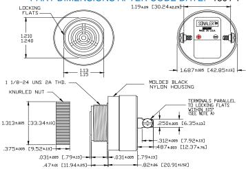
NOTE A: TERMINALS-.032 BRASS TIN PLATED, TAPPED FOR #6-32 SCREW, TWU #6-32 NICKEL PLATED BRASS SCREWS INCLUDED, WILL ACCEPT 1/4\* QUICK CONNECT. NOTE B: MOUNTING- REMOVE BLACK PLASTIC NUT AND INSERT THREADED FRONT THREUGH 1.25' HOLE PUNCHED IN PANEL, IF DRIENTATION IS NEEDED, NOTE LOCKING FLATS ON DRAWING. SCREW NUT BACK ON. DO NOT OVERTIGHTEN.
