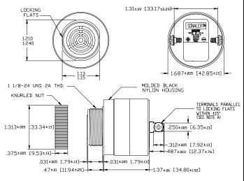
NOTE A TERMINALS-032 BRASS TIN PLATED, TAPPED FOR #6-32 SCREW. TWO #6-32 NICKEL PLATED BRASS SCREWS INCLUBED. WILL ACCEPT 1/4' QUICK CONNECT. NOTE B: MOUNTING- REMOVE BLACK PLASTIC NUT AND INSERT THREADED FRONT THROUGH 1.25' HOLE PUNCHED IN PANEL, IF DRIENTATION IS NEEDED, NOTE LOCKING FLATS ON DRAVING. SCREW NUT BACK ON. DO NOT OVERTIGHTEN.
