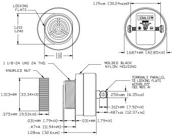
NOTE A: TERMINALS-032 BRASS TIN PLATED, TAPPED FOR #6-32 SCREW. TWO #6-32 NICKEL PLATED BRASS SCREWS INCLUDED. WILL ACCEPT 1/4\* QUICK CONNECT. B: MOUNTING- REMOVE BLACK PLASTIC NUT AND INSERT THREADED FRONT THROUGH 1.25' HOLE PUNCHED IN PANEL, IF ORIENTATION IS NEEDED, NOTE LOCKING FLATS ON DRAWING SCREW NUT BACK ON. DO NOT OVERTIGHTEN.
