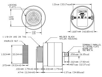
NOTE A: TERMINALS-032 BRASS TIN PLATED, TAPPED FOR #6-32 SCREW. TWO #6-32 NICKEL PLATED BRASS SCREWS INCLUBED. WILL ACCEPT 1/4' QUICK CONNECT. NOTE B: MOUNTING- REMOVE BLACK PLASTIC NUT AND INSERT THREADED FRONT THROUGH 1.25' HOLE PUNCHED IN PANEL, IF ORIENTATION IS NEEDED, NOTE LOCKING FLATS ON DRAVING. SCREW NUT BACK ON. DO NOT OVERTIGHTEN.
