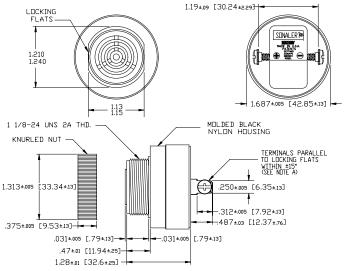
NOTE A: TERMINALS-032 BRASS TIN PLATED, TAPPED FOR #6-32 SCREW. TWO #6-32 NICKEL PLATED BRASS SCREWS INCLUBED. WILL ACCEPT 1/4' QUICK CONNECT. NOTE B: MOUNTING- REMOVE BLACK PLASTIC NUT AND INSERT THREADED FRONT THROUGH 1.25° HOLE PUNCHED IN PANEL, IF ORIENTATION IS NEEDED, NOTE LOCKING FLATS ON DRAVING. SCREW NUT BACK ON. DO NOT OVERTIGHTEN.
