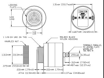
NOTE A: TERMINALS-.032 BRASS TIN PLATED, TAPPED FOR #6-32 SCREW. TWD #6-32 NICKEL PLATED BRASS SCREWS INCLUDED. WILL ACCEPT 1/4\* QUICK CONNECT. NOTE B: MOUNTING- REMOVE BLACK PLASTIC NUT AND INSERT THREADED FRONT THROUGH 1.25' HOLE PUNCHED IN PANEL, IF DRIENTATION IS NEEDED, NOTE LOCKING FLATS ON DRAWING, SCREW NUT BACK ON. DO NOT DVERTIGHTEN.
