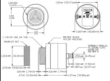
NOTE AF TERMINALS-032 BRASS TIN PLATED, TAPPED FOR #6-32 SCREW. TWO #6-32 NICKEL PLATED BRASS SCREWS INCLUBED. WILL ACCEPT 1/4' QUICK CONNECT.
