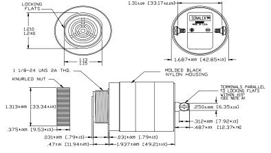
NOTE A: TERMINALS-.032 BRASS TIN PLATED, TAPPED FOR #6-32 SCREW. TWO #6-32 NICKEL PLATED BRASS SCREWS INCLUDED. WILL ACCEPT 1/4\* QUICK CONNECT. NOTE B: MOUNTING- REMOVE BLACK PLASTIC NUT AND INSERT THREADED FRONT THROUGH 1.25' HOLE PUNCHED IN PANEL, IF DRIENTATION IS NEEDED, NOTE LOCKING FLATS ON DRAWING, SCREW NUT BACK ON. DO NOT OVERTIGHTEN.
