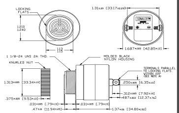
NOTE A: TERMINALS-032 BRASS TIN PLATED, TAPPED FOR #6-32 SCREW. TWO #6-32 NICKEL PLATED BRASS SCREWS INCLUBED. WILL ACCEPT 1/4' QUICK CONNECT. NOTE B: MOUNTING- REMOVE BLACK PLASTIC NUT AND INSERT THREADED FRONT THROUGH 1.25' HOLE PUNCHED IN PANEL, IF DRIENTATION IS NEEDED, NOTE LOCKING FLATS ON DRAWING, SCREW NUT BACK ON. DO NOT DVERTIGHTEN.
